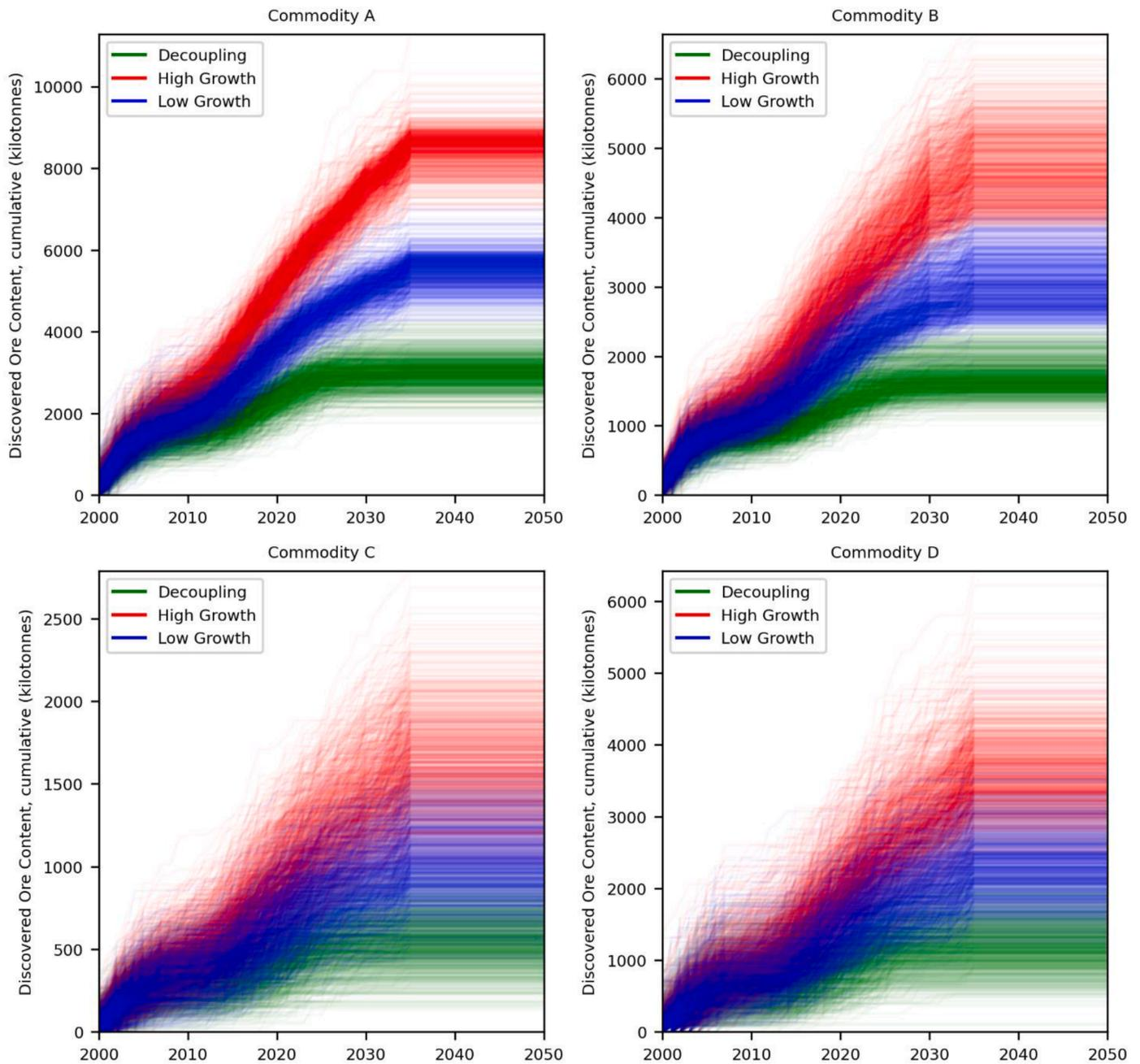
Fig. 5. Cumulative discovered ore content for a hypothetical 4 co-product commodity system (A, B, C & D), where demand for A and B must always be met. Results for three demand scenarios are shown, with 1000 iterations of the model run.
