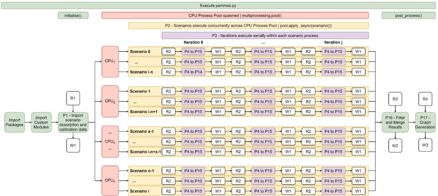
Fig. 3. Model execution flowchart as implemented in python (PEMSS v1.0.0), showing concurrent processing through the assignment of individual scenarios to a pool of (n) CPU processes. Iterations (j) execute sequentially within each scenario (i) to preserve random seeds and ensure reproducibility of results. Unit process abbreviations and colours correspond to those presented in Fig. 1.
