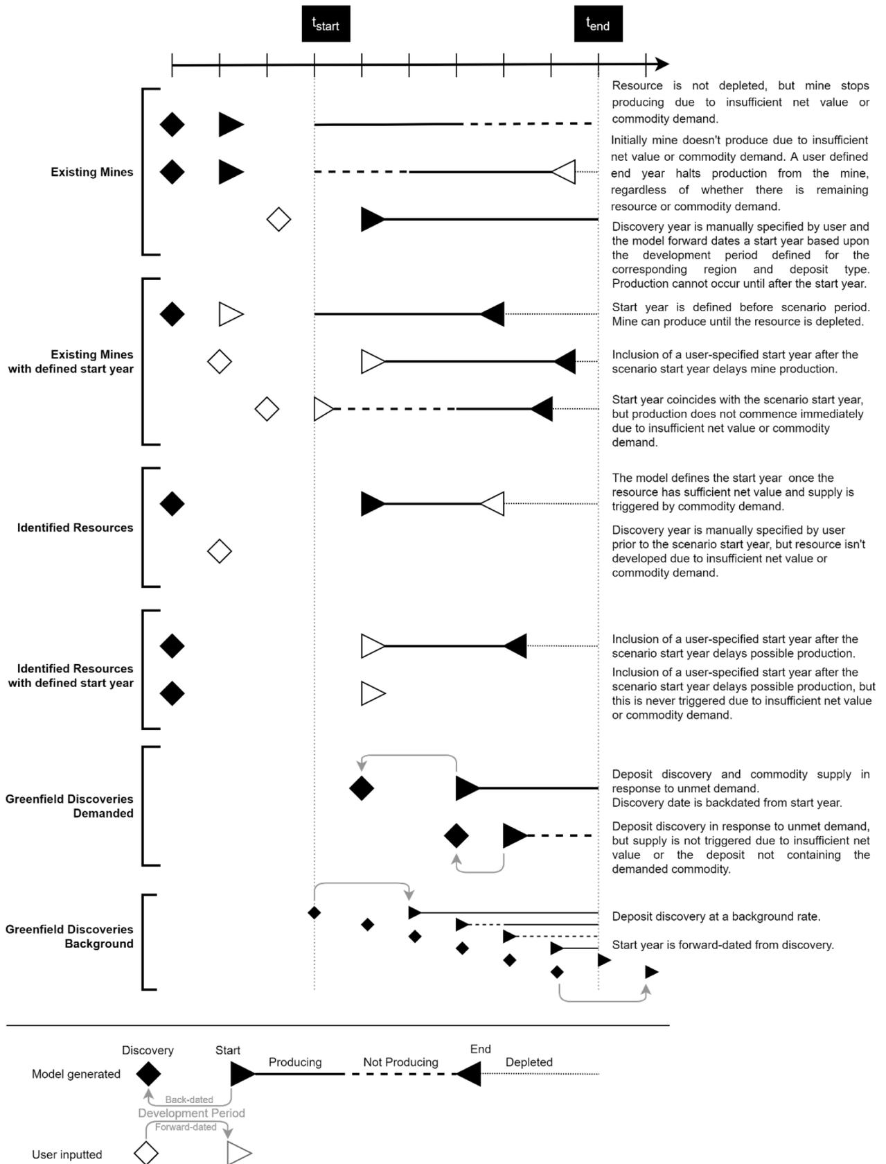
Fig. 2. Examples of possible mine behaviours and how this can be influenced by user-inputted information. The mine/resource categories on the left-hand side are referred to as ‘aggregations’ in model output files to enable summary statistics to be generated for specific cohorts of mines and deposits.
