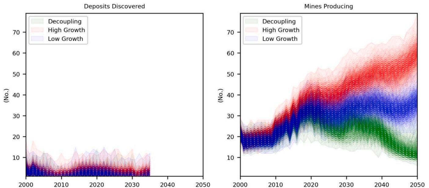
Fig. 6. Annual deposit discoveries and mines producing for a hypothetical 4 co-product commodity system. Results for three demand scenarios are shown, with 1000 iterations of the model run.
