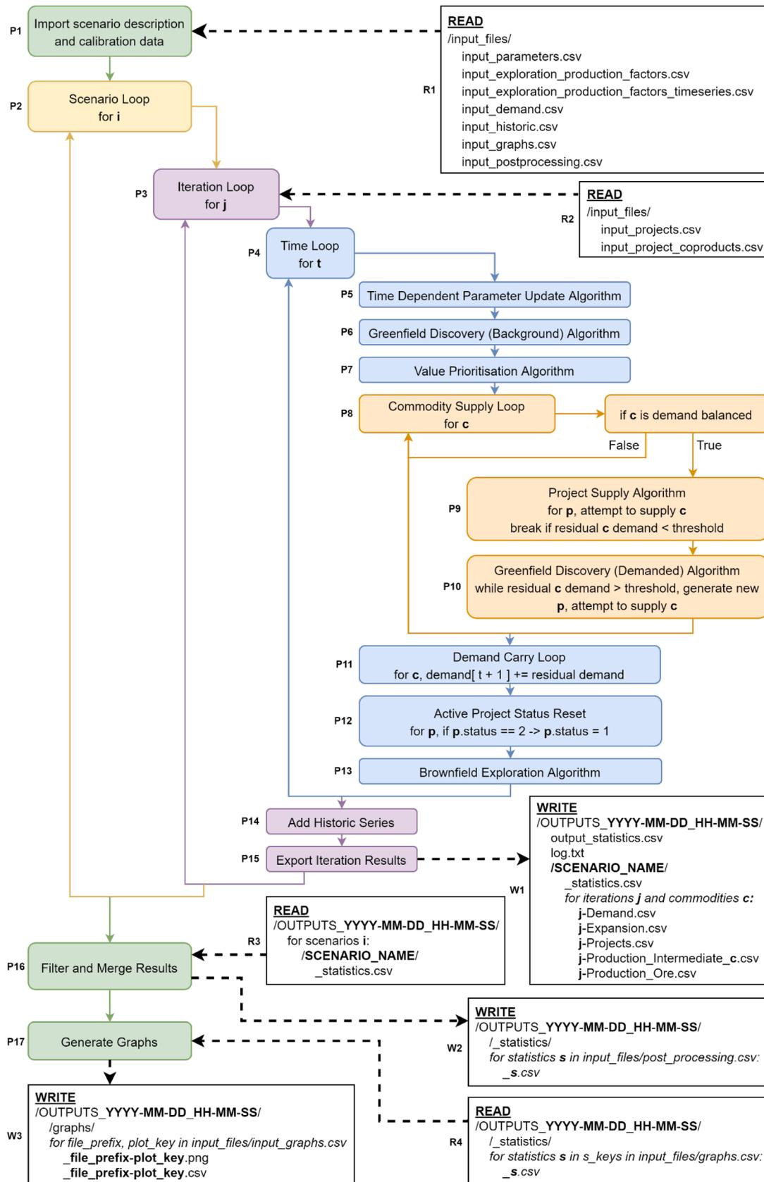
Fig. 1. PEMSS model flowchart of key algorithms and data exchanges. Abbreviations (e.g. P13, W1, R2, etc.) are cross-references and searchable within the model's python code that is available on GitHub and Zenodo (Northey et al., 2022).
