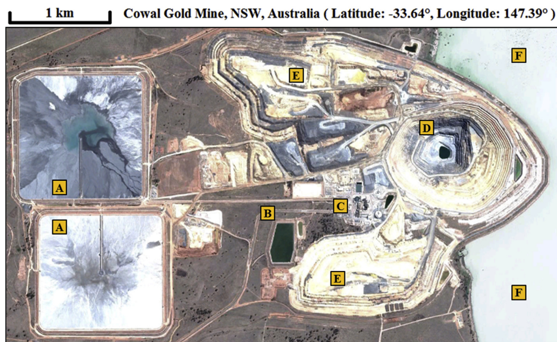
Fig. 2. Satellite image of Cowal Gold Mine located adjacent to Lake Cowal, New South Wales, Australia (Google Earth, 2016). Key points of interest are shown by the letter annotations: A – Tailings Storage Facilities, B – Water Storage, C – Ore Processing Facilities, D – Open Pit Mine, E – Waste Rock Dumps, F – Lake Cowal.
