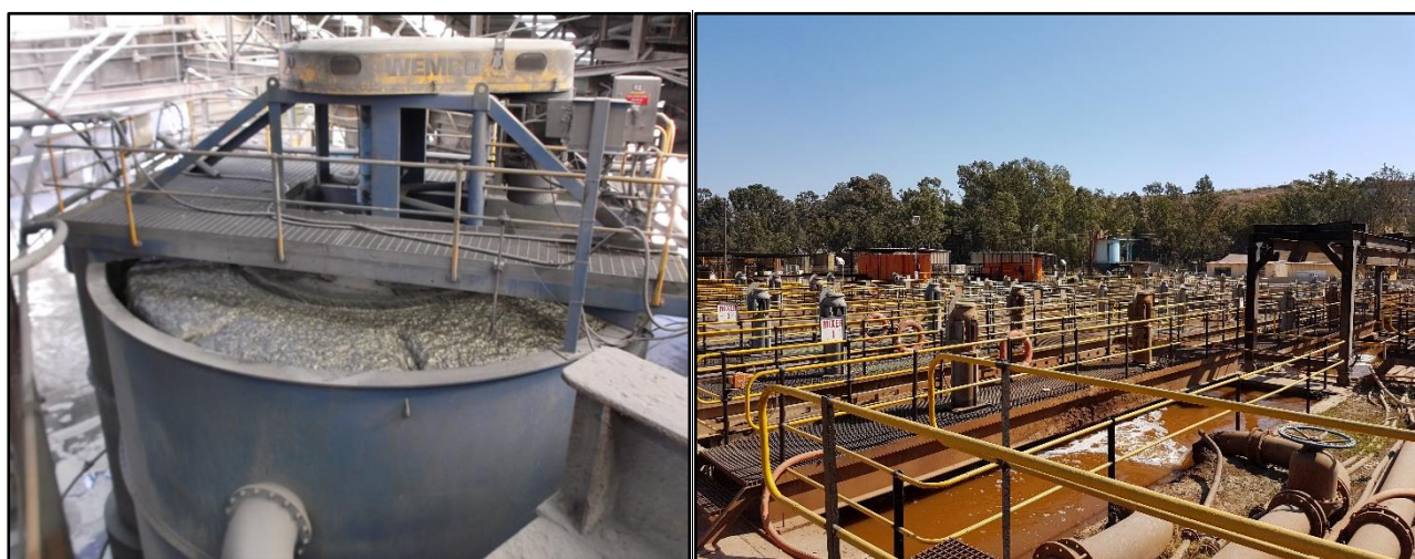
Figure 7.3: Examples of mineral separation and waste treatment processes. (Left) A 150m 3 flotation tank used in the initial ‘rougher’ separation of a copper concentrate from gangue mineralogy. Photo taken in March 2013 by the author (S.A. Northey). (Right) Aeration and settling tanks used for the treatment of acid mine drainage. Photo taken in August 2016 by the author (S.A. Northey).
